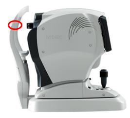
The patient's eyes should be aligned with the eye level markers on the side of the forehead rest support.
