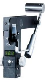
U type tonometers remain attached to Zeiss/Lower illumination style slit lamps, rotating in and out of position when needed.
