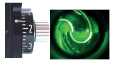
The measurement dial and probe position should be adjusted to reach the correct end point. The appearance of the mires will guide the adjustment needed:
