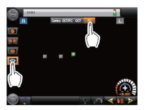
Before anterior image can be captured, anterior mode must be selected, and the compensation lens adjusted to the '+' position.
