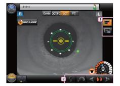
It is possible to use the touch screen of the device to manually move the fixation point to any preferred position. This feature can be used for single capture of images in peripheral location eg. Photography of a peripheral naevus.
