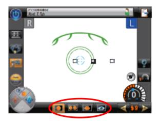
The different photography modes can be accessed at the bottom of the touch screen on the AFC 330.
