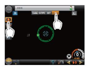
The 3 fixation points allow the centration of different retinal features during image capture.
